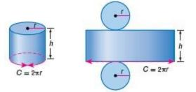
The surface area of this cylinder is  $2\pi r h + 2\pi r^2$ .
